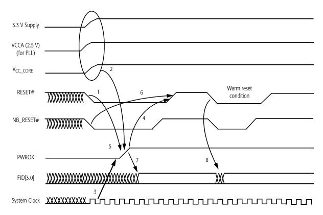
Figure 11. Signal Relationship Requirements During Power-Up Sequence
