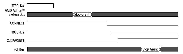
Figure 3. AMD Athlon™ System Bus Disconnect Sequence in the Stop Grant State
