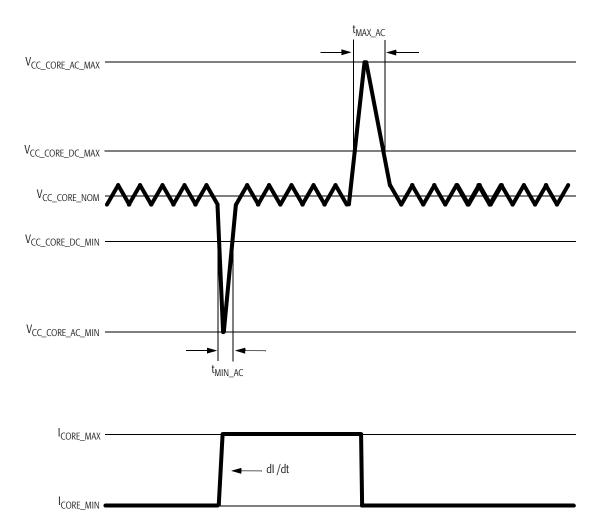
Figure 7. V<sub>CC CORE</sub> Voltage Waveform
