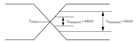
Figure 8. SYSCLK and SYSCLK# Differential Clock Signals
